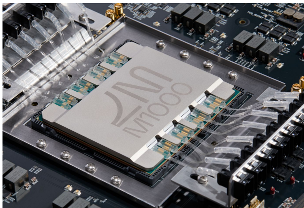
Multi-reticle 3D stacked CPO with fiber array connectivity (M1000)
